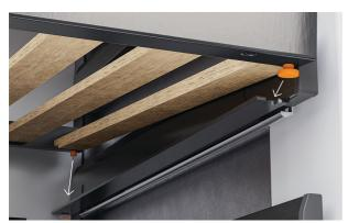
**3.** To refit, push the front pins into the slide support and lower the rack until the rear pins lock into place.
